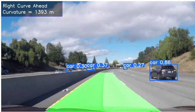
Fig. 15: Integration of Lane and Vehicle Detection
