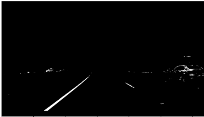
Fig. 6: Combining H and S Threshold
